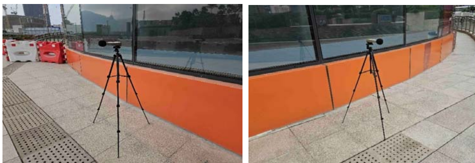
The station set-up of a façade measurement at station NM2A.
