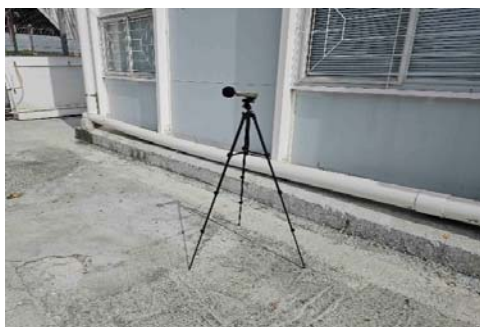
The station set-up of a façade measurement at station NM4A.
