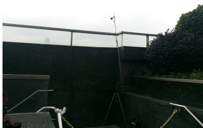
The station set-up of a free-field measurement at Station NM1A.
