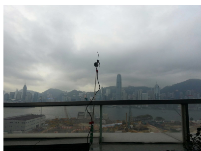
The station set-up of a free-field measurement at Station NM1A.
