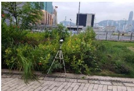
The station set-up of a free-field measurement at station NM5A.
