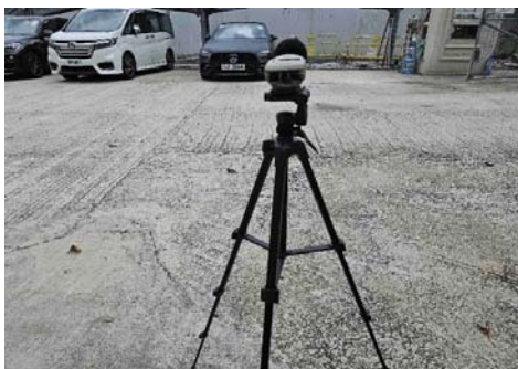
The station set-up of a façade measurement at station NM4A.
