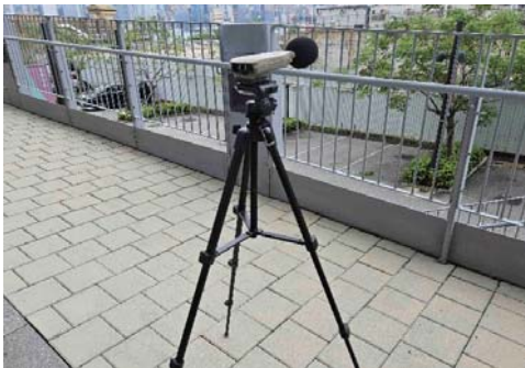
The station set-up of a façade measurement at station NM3A.
