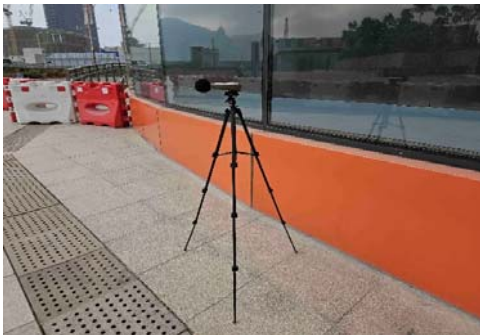
The station set-up of a façade measurement at station NM2A.
