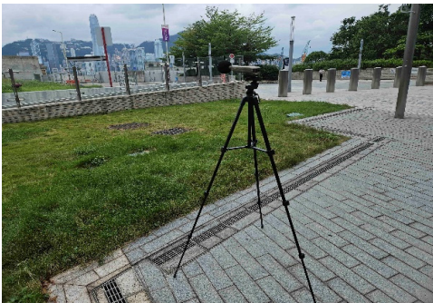
The station set-up of a free-field measurement at station NM5A.
