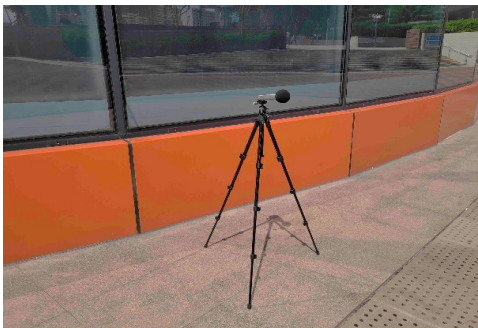
The station set-up of a façade measurement at station NM2A.
