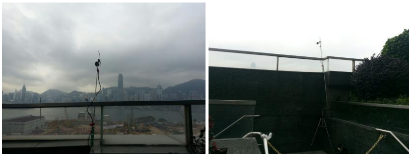
The station set-up of a free-field measurement at Station NM1A.
