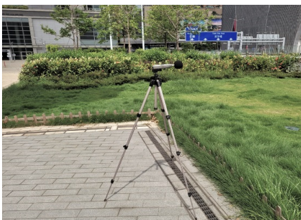
The station set-up of a free-field measurement at station NM5A.
