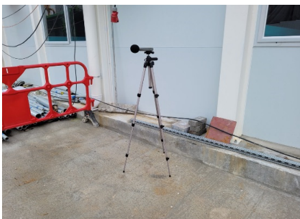
The station set-up of a façade measurement at station NM4A.
