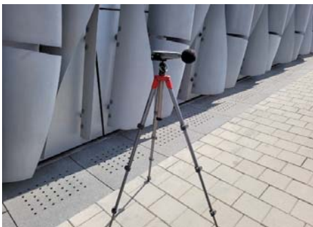
The station set-up of a façade measurement at station NM3A.
