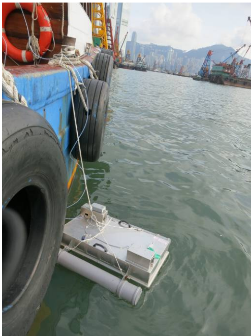
Photo 3.7 Floating ventilated sampling hood on the sea surface
