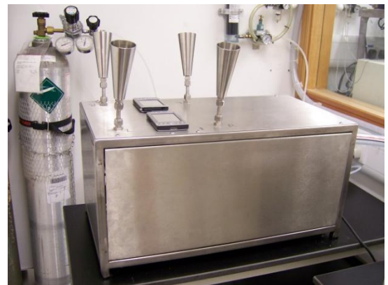
Figure 3 - Olfactometer (Oldacton-n2) at Odour Lab
