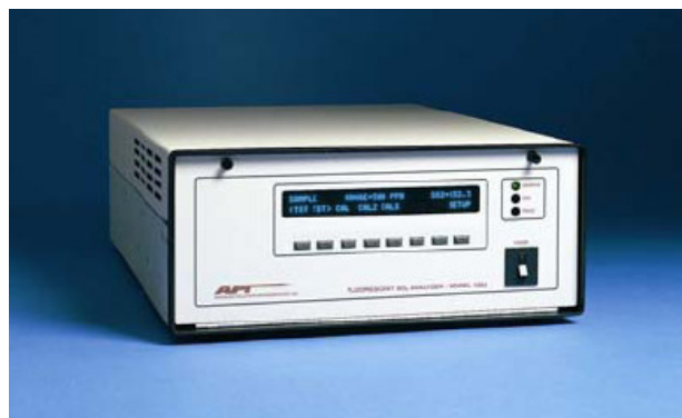
Photo 2.6 TeledynAPI Model 101E desktop UV fluorescence H 2 S analyzer
